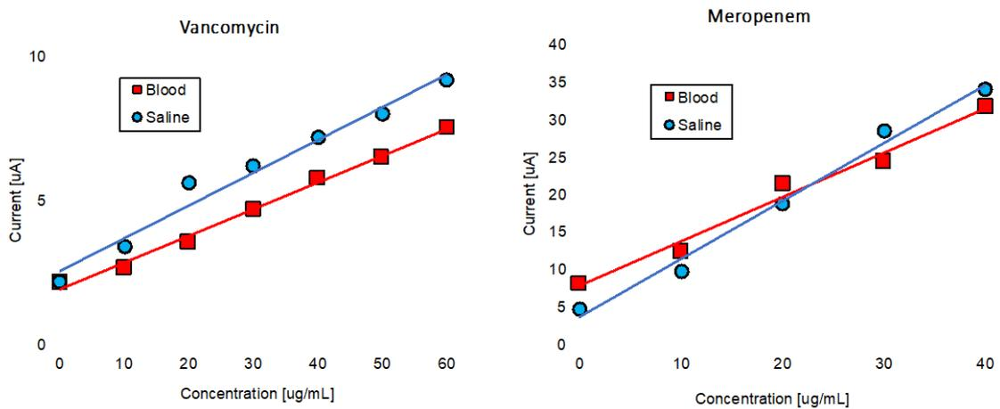
**Fig. 2:** Calibration curve of vancomycin and meropenem by the respective MIP-sensor chip.
