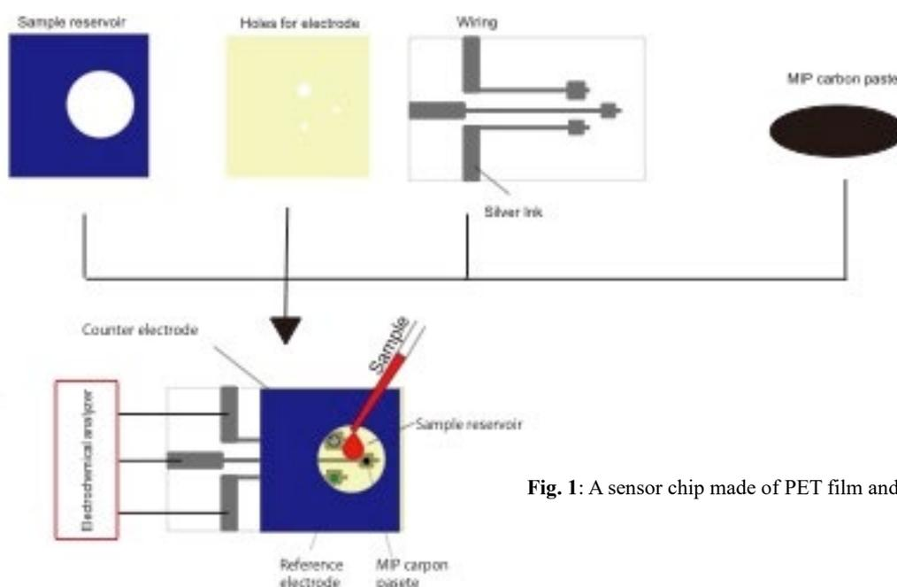
**Fig. 1:** A sensor chip made of PET film and MIP carbon paste
